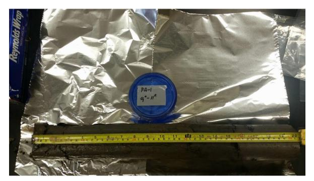
**PHOTOGRAPH 2** Fly Ash Pond Undisturbed Soil Sample FA-1.
