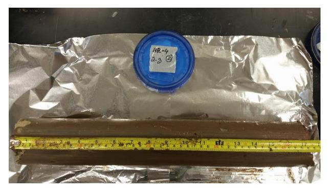
**PHOTOGRAPH 5** Bottom Ash Pond Undisturbed Soil Sample AB–4.
