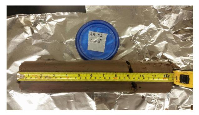
**PHOTOGRAPH 2** Bottom Ash Pond Undisturbed Soil Sample AB-1.
