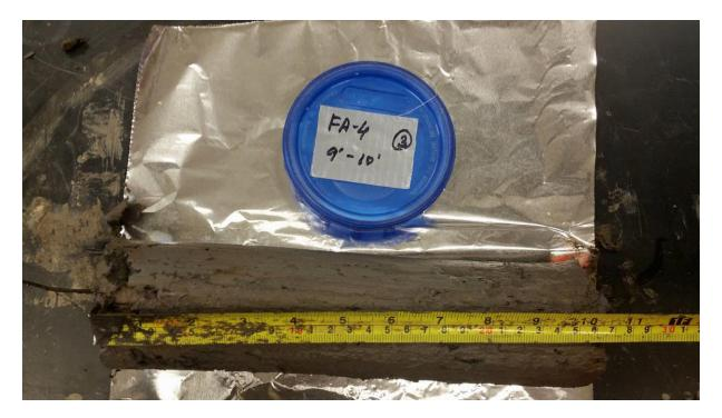
**PHOTOGRAPH 5** Fly Ash Pond Undisturbed Soil Sample FA-4.
