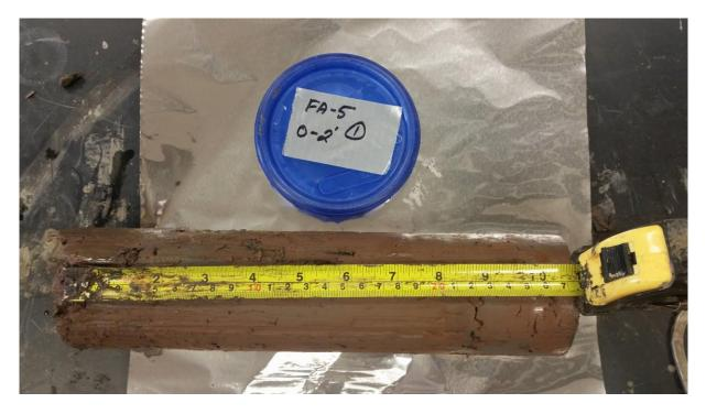
**PHOTOGRAPH 6** Fly Ash Pond Undisturbed Soil Sample FA-5.
