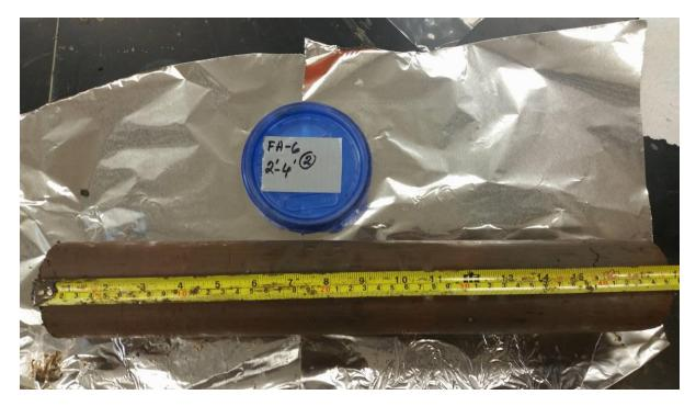
**PHOTOGRAPH 7** Fly Ash Pond Undisturbed Soil Sample FA-6.
