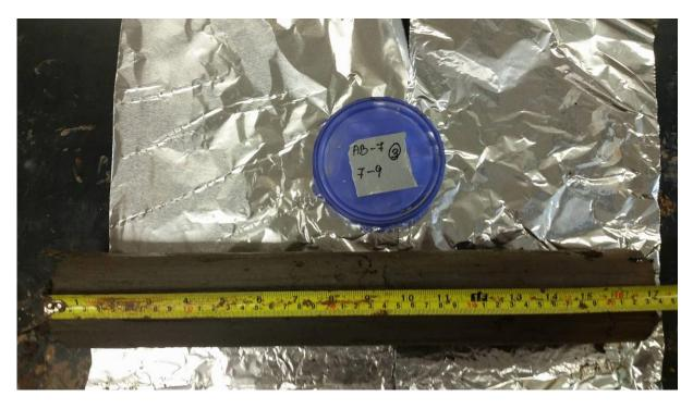
**PHOTOGRAPH 8** Bottom Ash Pond Undisturbed Soil Sample AB–7.
