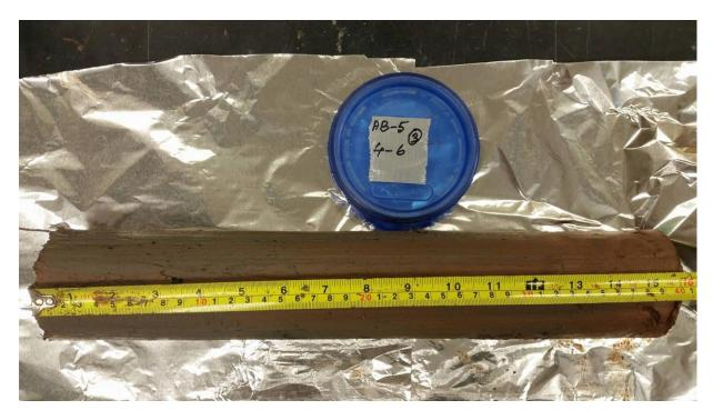
**PHOTOGRAPH 6** Bottom Ash Pond Undisturbed Soil Sample AB–5.
