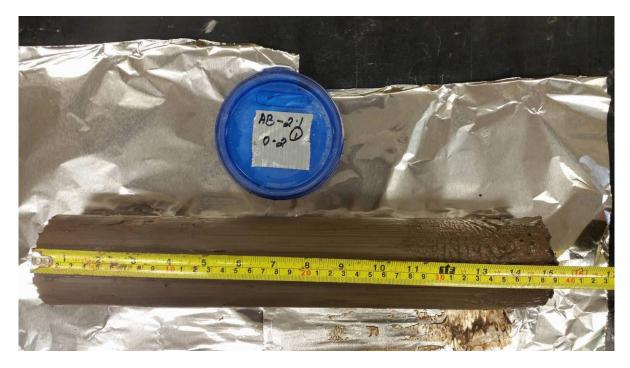
**PHOTOGRAPH 3** Bottom Ash Pond Undisturbed Soil Sample AB–2.
