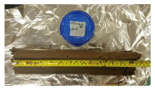
**PHOTOGRAPH 7** Bottom Ash Pond Undisturbed Soil Sample AB–6.
