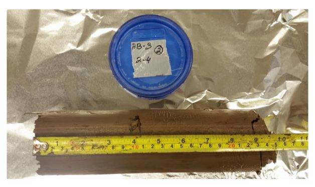
**PHOTOGRAPH 4** Bottom Ash Pond Undisturbed Soil Sample AB–3.
