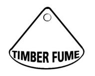
This tag is an example of a fumigant treatment tag. This tag shall be used whenever MITC-FUME or DuraFume or Woodfume or TimberFume (Select One) is applied to a pole. This tag will be used in conjunction with one of the above tags depending on the type of inspection performed.
