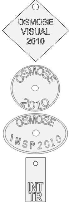
This diamond shaped tag represents that a visual inspection **only** was performed. This tag shows CONTRACTOR's name, identifies that a visual inspection was performed, and the actual year the work is performed.
